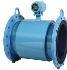
Magnetic bi-directional flowmeter with stainless steel electrodes, 4-20 mA output local display, NEMA4X housing, and no moving parts to wear out
