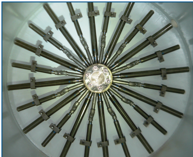
Common 304SS inlet/outlet design for Packed Bed
