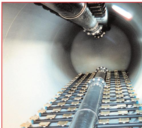
*Internal view of a horizontal filter with the underdrain installed prior to shipment.*
