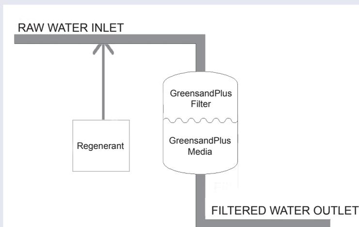
Catalytic Oxidation (CO) operation is recommended in applications where iron removal is the main objective in well waters with or without the presence of manganese. This method involves the feeding of a predetermined amount of chlorine ( $\text{Cl}_2$ ) or other strong oxidant directly to the raw water before the GreensandPlus Filter.
